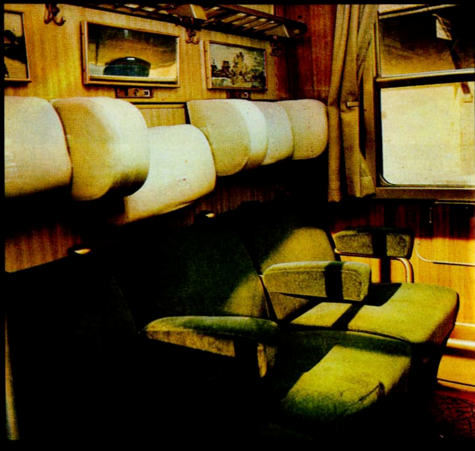
Suitable for speeds up to 200 k.p.h.. Length 26.40 m., tare 41 tons, high-speed brake. 10 compartments with 60 seats, seats in sponge rubber, fluorescent lighting, steam and electric heating with thermostat control in each compartment.
